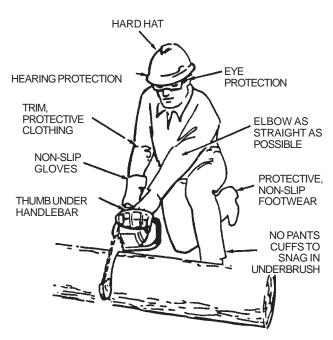
Fig. 1 - Correct Protective Articles, Grip, and Positioning
